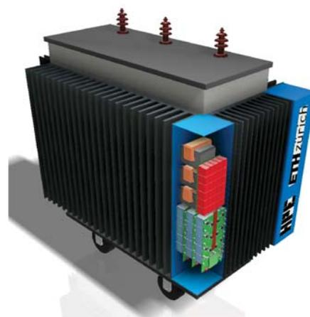
Figure 18: 3D rendering of the 400kVA HT visualizing the volume increase caused by the converter.
